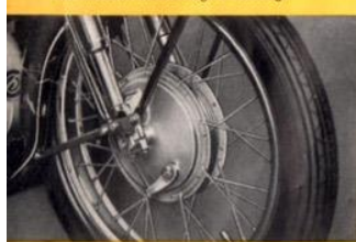
Hoffmann aluminium hub with internal expanding brake
