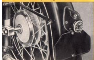
Rear hub with telescopic springing.
